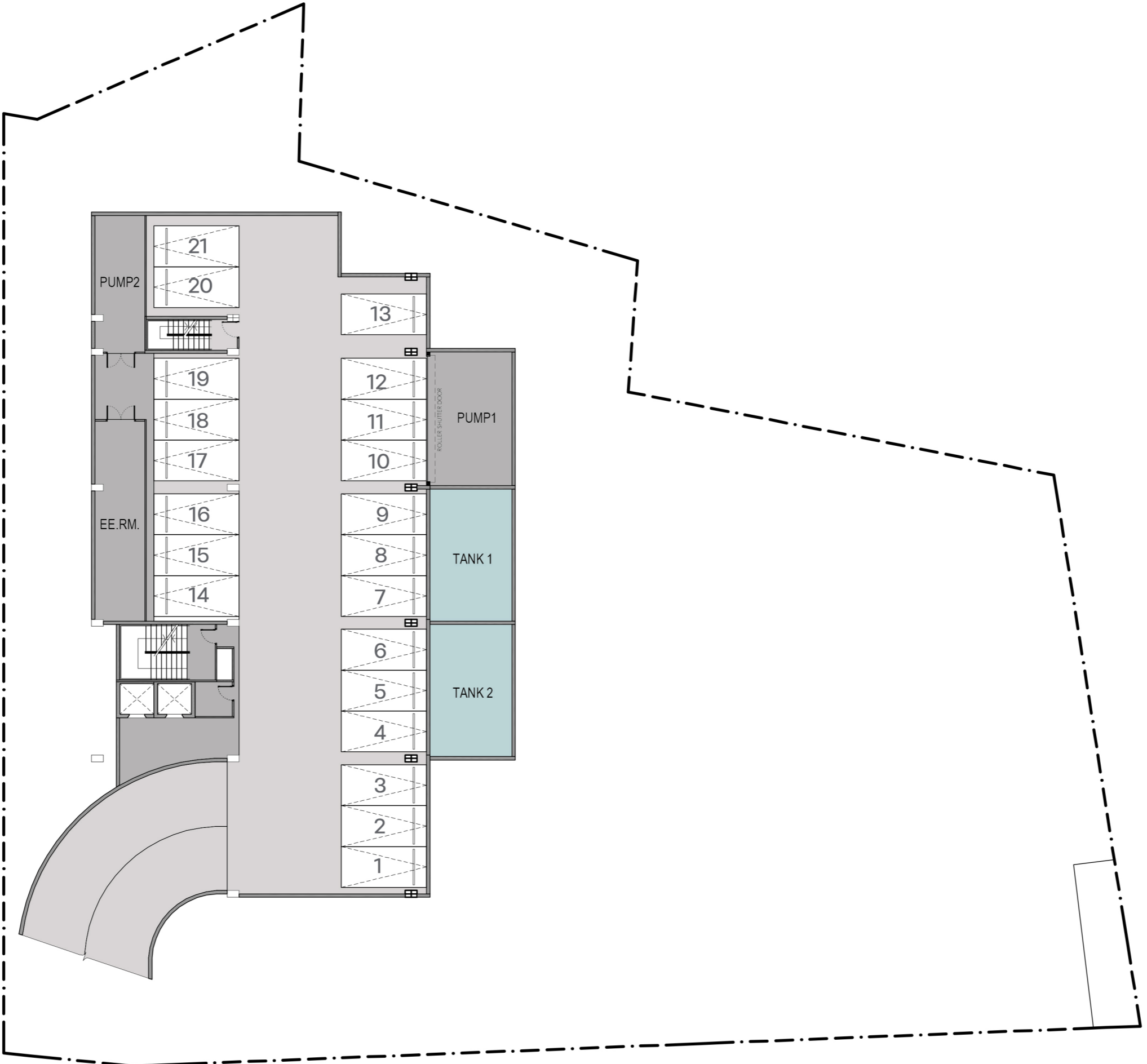
BASEMENT LAY-OUT PLAN BUILDING K1-K2
